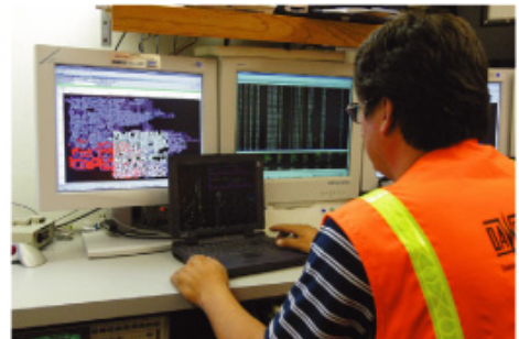
Technician operating a seismic recording system.
