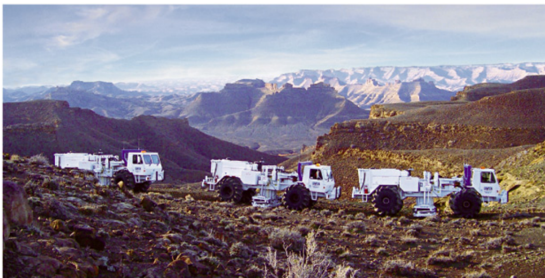
Vibrator energy source units operating in Utah.
