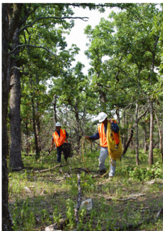
Crew deploying geophones and cables.
