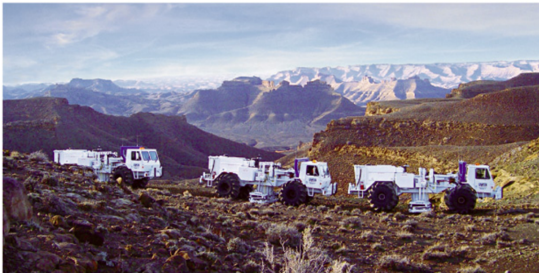
Vibrator energy source units operating in Utah.
