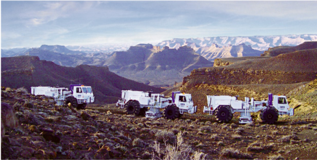
Vibrator energy source units operating in Utah.
